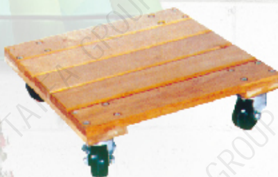
T0525 (TC0514-I) Own Weight(kg):5.6 Load Capacity(kg):300 Wheel:3" Body Size ( LxWxH)(mm): 450x450x135
