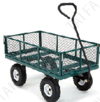
TC1849 Own Weight(kg):33.6 Load Capacity(kg):350 Pneumatic Tyre:3.50-4 Body Size ( LxWxH)(mm): 1100x510x1100
