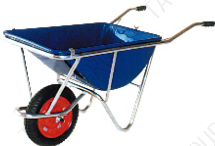
WB2204-1 Load Capacity(kg):100 Own Weight(kg):12.3 Water capacity(L):60 Sand Capacity(CBF):5 Wheel:13 " x3 " L/H/C(mm):1245x615x615 A/B/h(mm):775x495x280
