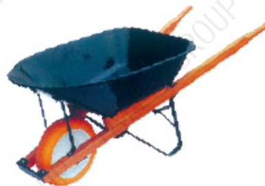
WH7611 Load Capacity(kg):200 Own Weight(kg):21 Water capacity(L):90 Sand Capacity(CBF):7 Wheel:4.00-8 L/H/C(mm):1605x585x645 A/B/h(mm):1030x675x280
