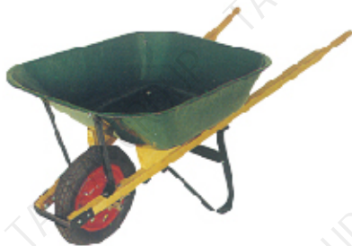
WH6202 Load Capacity(kg):130 Own Weight(kg):10 Water capacity(L):65 Sand Capacity(CBF):5 Wheel:13" x3" L/H/C(mm):1340x540x520 A/B/h(mm):820x660x210
