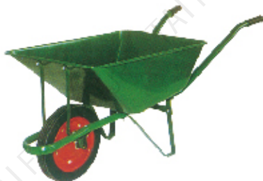
WB2500 Load Capacity(kg):120 Own Weight(kg):12.4 Water capacity(L):60 Sand Capacity(CBF):5 Wheel:13 " x3 " L/H/C(mm):1310x550x490 A/B/h(mm):775x500x230
