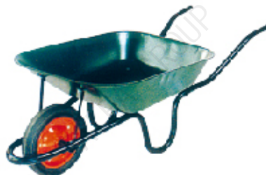
WB3800 Load Capacity(kg):100 Own Weight(kg):12.7 Water capacity(L):60 Sand Capacity(CBF):4 Wheel:13 " x3 " L/H/C(mm):1380x540x450 A/B/h(mm):830x615x255
